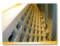
Heavy reinforced **grate** frame with a two inch thick 500 BHN rebuildable liner. Optional hole patterns are available for different applications and end-product requirements.
