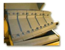
A patented, high inertia solid steel **rotor** with four alternating angled rows of striker bars ensures even distribution of material being processed for balanced wear and maximum throughput.
