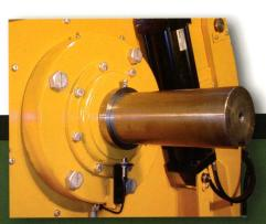
Extra heavy duty **swing away anvil** with bolt-on liner for ease of replacement.
