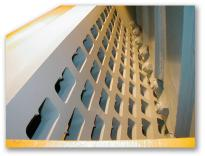
Heavy reinforced **grate** frame with a 500 BHN rebuildable liner. Optional hole patterns are available for different applications and end-product requirements
