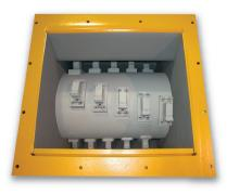
High inertia steel **rotor** with alternating rows of fang tooth stikers ensures even distribution of material being processed for balanced wear and maximum throughput.
