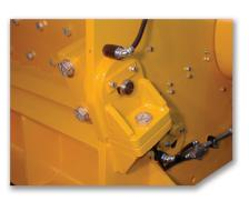
Grate, anvil, and upper frame are **electronically interlocked** to ensure maintenance personnel safety as well as remote monitoring during operation.
