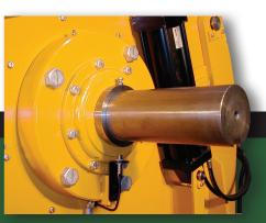
Extra heavy duty **swing away anvil** with bolt-on liner for ease of replacement.
