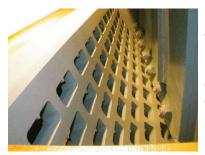
Heavy reinforced **grate** frame with a two inch thick 500 BHN rebuildable liner. Optional hole patterns are available for different applications and end-product requirements.
