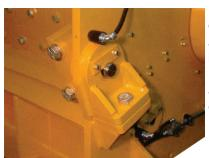
Grate, anvil, and upper frame are **electronically interlocked** to ensure maintenance personnel safety as well as remote monitoring during operation.
