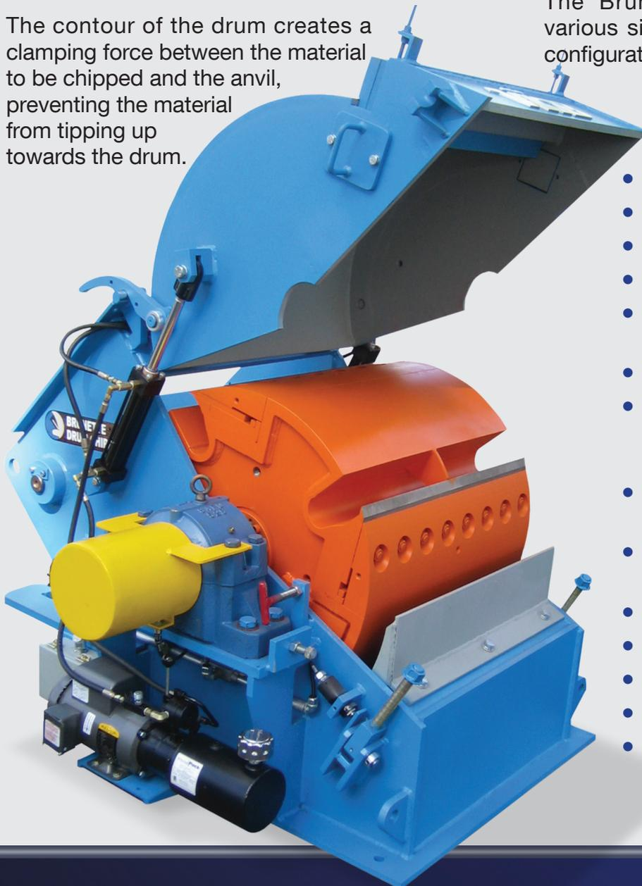
The Drum Chipper is equipped with a clam shell opening operated by a hydraulic cylinder to give an ergonomically friendly working area for knife changes, which can be done quickly and easily by one person.
