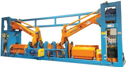
The custom designed dual head model allows for smooth flare butt removal regardless of log orientation.
