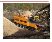
All DH series whole-tree chippers are standard-equipped with fluid coupling power transfer to eliminate clutch failure, hydraulically adjusted blower for ease of loading, and hydraulic door access for easy blade changes. With the standard electric-hydraulic pump, many system functions can be run for maintenance without engaging the DaimlerChrysler OM502 LA engine.
