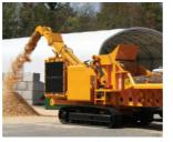
or end loading of trailers, and also features both a hydraulic blower for stronger chip discharge, which increases power when needed, and an actuated chip deflector. The ChipMax is available as a portable [pintle hook or fifth wheel mounting hitch], track, or truck-mounted unit, and is road legal in both width and weight.
